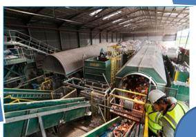
Next, it is transferred to a Materials Recovery Facility in St Albans. Magnets, air jets and large rotating drums are used to separate the recycling.
