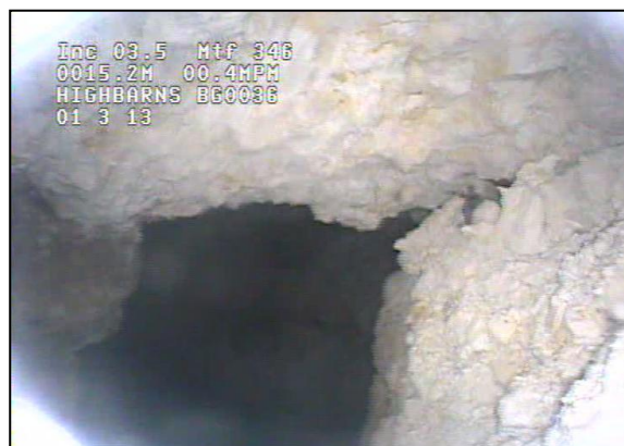
CCTV image of previously unidentified mine void on the corner of Highbarns/East Green
