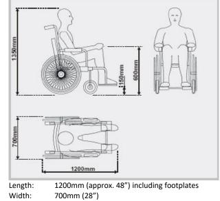
Width:700mm (28")Total seated height:1350mm (54")Clearance under footplate:150mm (6")
